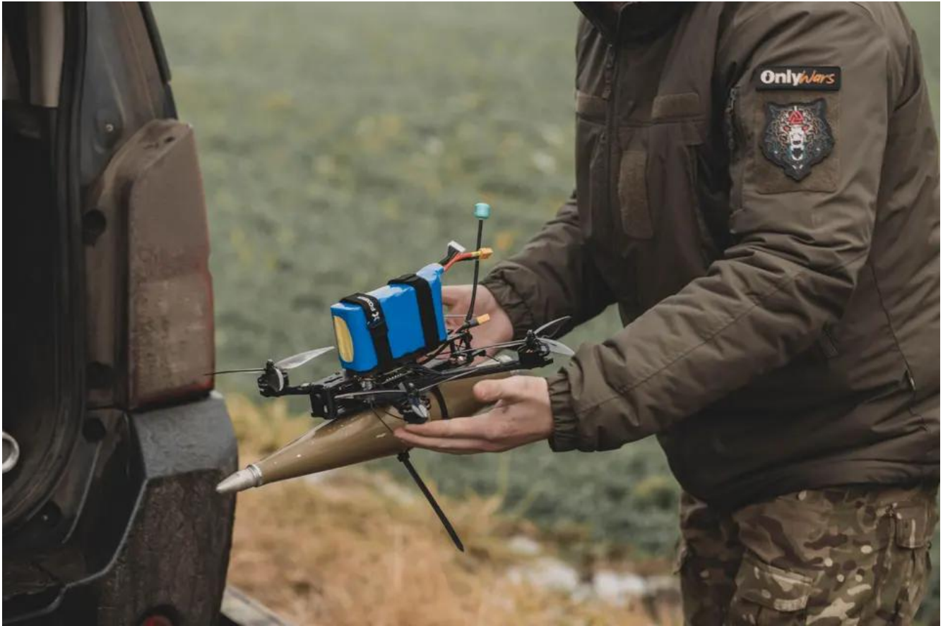
Figure 2: Ukrainian FPV (First Person View) attack drone equipped with a warhead and a system that carries out the final stage of the attack autonomously. (Forbes)
